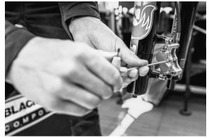
Bolt the front brake caliper to the fork's lower leg. This must be centered with the brake rotor once the wheel is installed.
