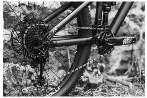
Fasten the dérailleur to the hanger, ensuring that they are aligned correctly (with b-tension screw in contact with the dérailleur's plastic washer rather than the hanger itself).
